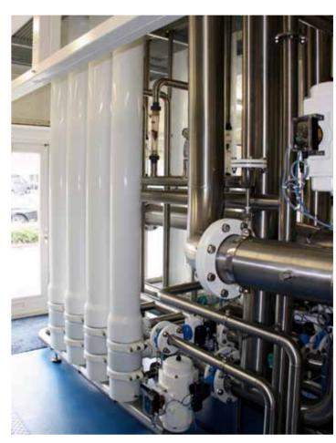
hospital wastewater. The Paques downstream membranes were compared to an upstream system with air injection from below. It appeared that the downstream membranes, with air intake from above, showed permeability twice as high for only a third of the energy consumption. Finally, the side-stream membrane installations as the BIOPAQ®MBR are inherently more hygienic than submerged membranes and the maintenance is easier and costs, especially with the new downstream membranes, much less time.
